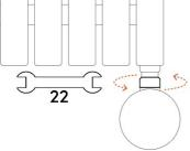
**NOTE** - Never attempt to tighten the element by twisting the control head or product housing. Always use the correct tools as directed in the instructions.
