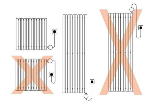
3. Tilt the radiator until the fitting location is at the highest point. This prevents any fluid escaping if your radiator is pre-filled.
