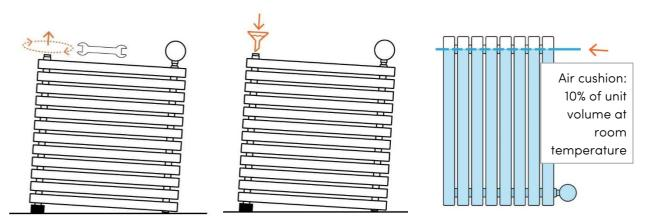
**NOTE** – It is critical that the correct volume of heating medium is used. Underfilling the radiator will impede circulation and prevent the unit from heating up. Overfilling the radiator can cause a dangerous build up of pressure as the fluid heats up. A suitable air cushion must be maintained. Calculating the volume of heating medium is a job for a professional electrician or heating engineer and should not be attempted DIY. If unsure, use the element only with a pre-filled radiator.
